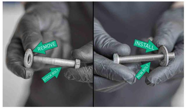
Install the factory spring, washer, new bolt, and new nut through the IE downpipe mount using a 13mm crescent wrench and 13mm socket.
