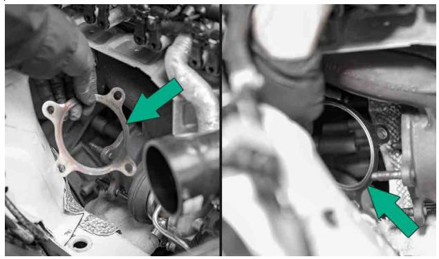
Install the new IE downpipe onto the turbo studs with the IE logo is facing upwards.
