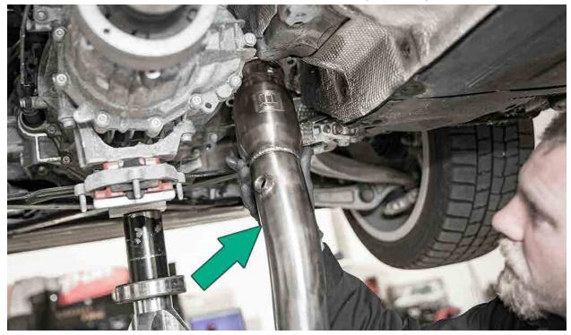
Reinstall the transmission mount and remove the jack support.
