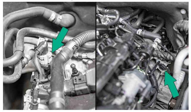
Using a 22mm wrench or 02 sensor tool, remove both 02 sensors from the stock downpipe.
