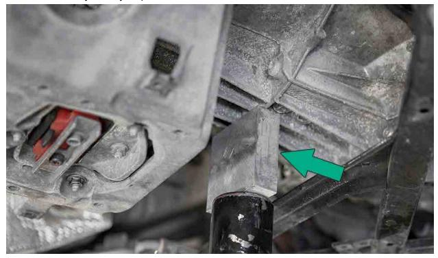
Remove the 4 outside transmission mount bolts with a triple square 12 bit. Remove the 3 inside bolts with a 13mm socket to release the transmission mount from the chassis.
