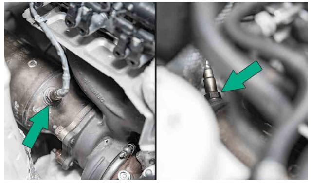
Remove the 4 CAT to turbo stud nuts with a 16mm socket.
