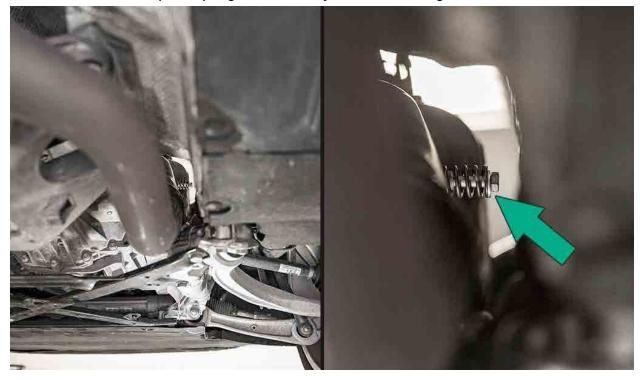
Remove the 3 nuts from the downpipe to midpipe flange with a 12mm crescent wrench.
