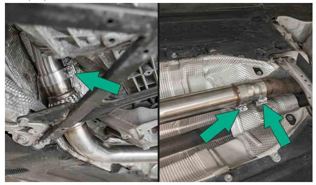
Reinstall the belly pan. Start your car and inspect for any exhaust leaks. After driving the car for 1-2 days verify all bolts, nuts, and clamps are tight.
