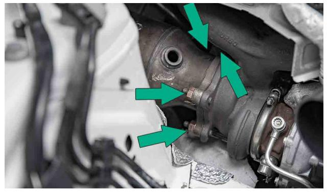
Using a 13mm socket, remove the bolt and washer from the spring mount on the downpipe. *Note: Make sure to keep the spring and washer, you will be reusing these for install.*
