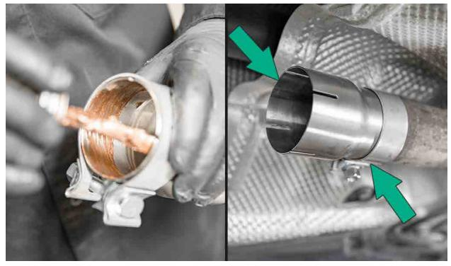
Place one large exhaust clamp over the slip-fit adapter. Note: Do not tighten clamps in this step.
