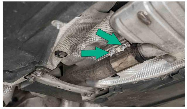
Remove the midpipe and rear exhaust clamp from the vehicle.
