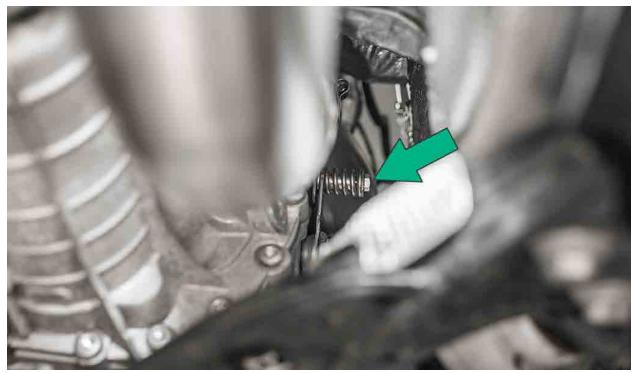
Place the new small exhaust clamp and slip-fit adapter onto the factory catback. Line all slip-fit ends with anti-seize. *Note: Do not tighten clamp in this step.*
