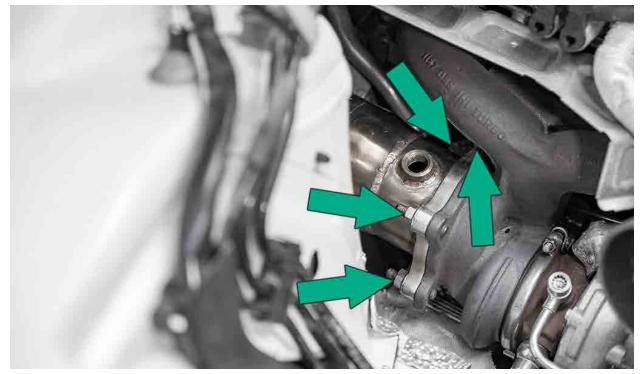
Coat the 02 sensor threads with anti-seize, then reinstall into the new IE downpipe. Plug the electrical clips back into the appropriate harness connectors.
