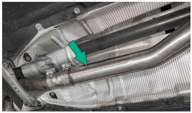
Adjust so that everything sits even, without binding, or drooping. Tighten all 3 exhaust clamps. *Note: Exhaust clamps need to be very tight, they must compress the tubing to fully seal slip-fits. The torque spec is 50 ft-lb.*
