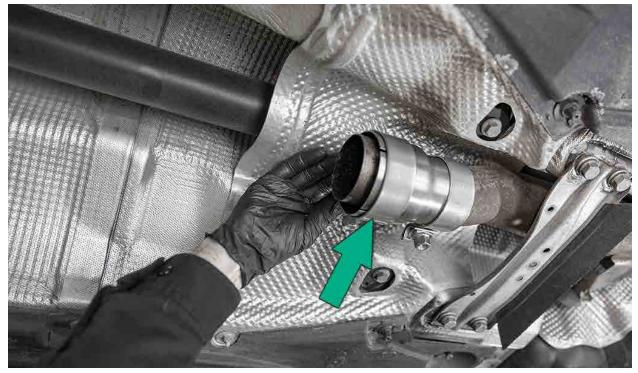
Place the remaining large exhaust clamp over the new IE midpipe.
