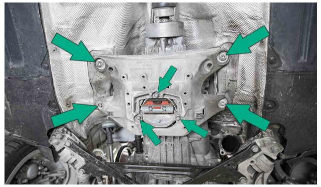
Remove the transmission mount to make room, then remove the factory downpipe.
