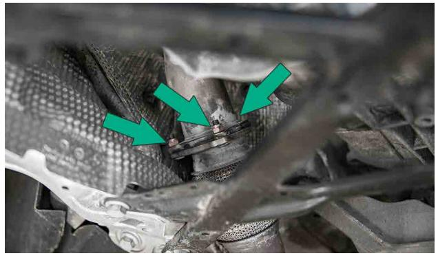
Remove the rear exhaust clamp nuts with a 13mm socket.
