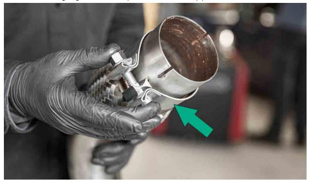
Install the midpipe into place between the downpipe section and catback fully seating the slip-fits on both ends. *Note: Do not tighten clamps in this step*.
