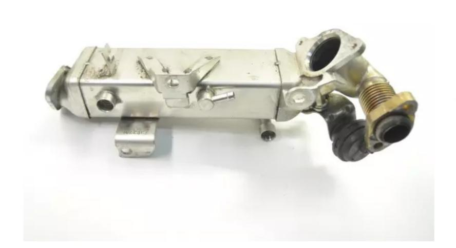
Remove complete EGR valve + EGR cooler + all piping Blank all ports.
