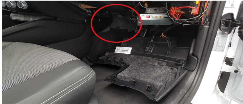
From No.9 - after trim removed, locate the CAN Gate connector.
