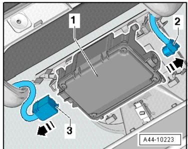
Unplug electrical connectors -2- and -3- and remove camera control unit -J852--1-
