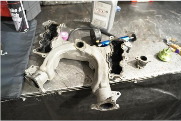
1 Blanking plate will be installed between the inlet manifold and short joining pipe (shown below)
