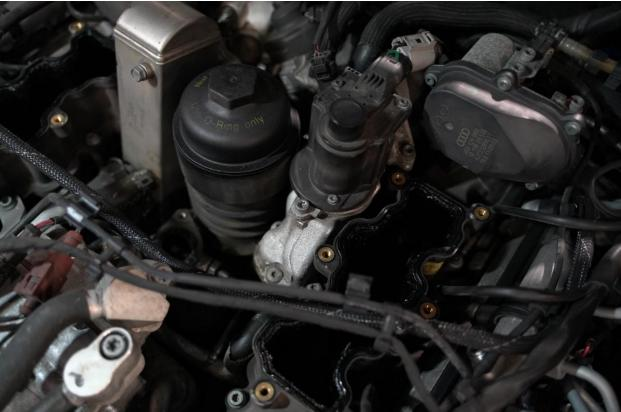
The remaining 2 blanking plates are installed on the head. The stock sensors are retained.
